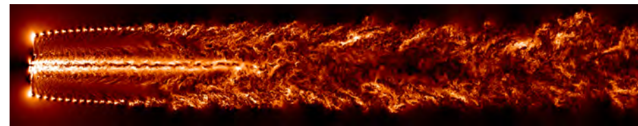
Instantaneous axial momentum at multiple downstream positions of the National Renewable Energy Laboratory WindPACT-1.5MW wind turbine.
