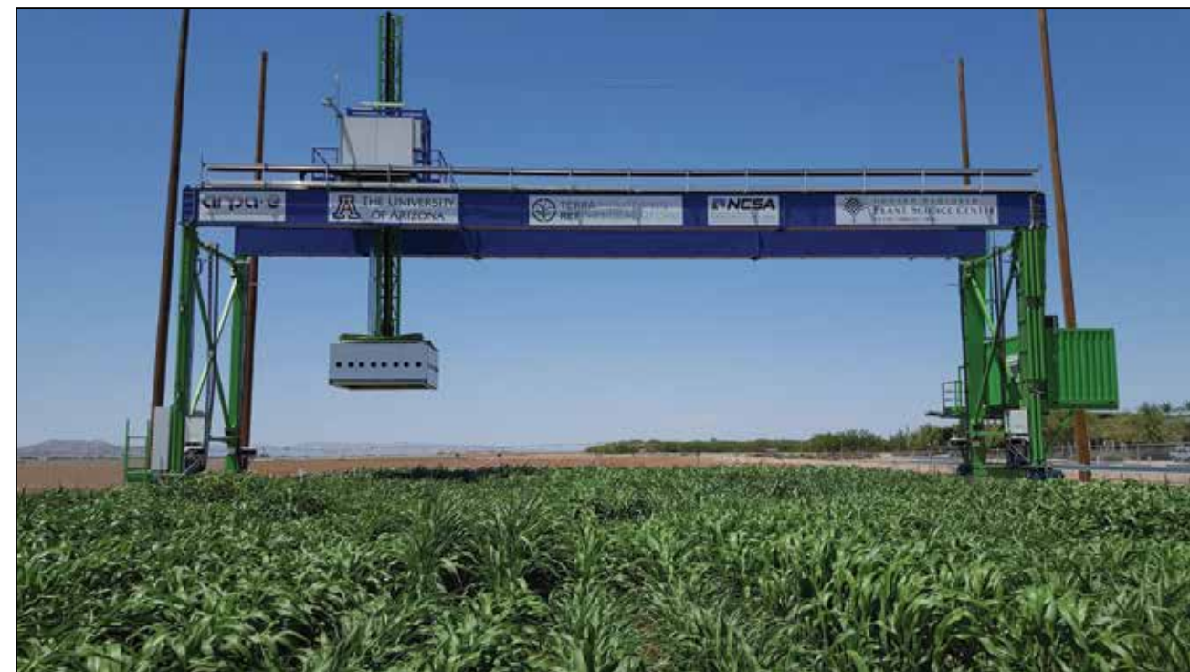
Figure 1: Field scanner system (with sensors in white box) operating on 200-meter steel rails in Maricopa, Arizona, U.S.A.
