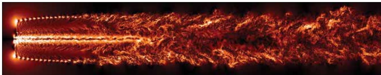
Figure 1: Wind turbine wake slice visualizing instantaneous normalized absolute tangential flow velocity demonstrating the wake propagation downstream of a small-scale rotor design with a two-meter diameter.
