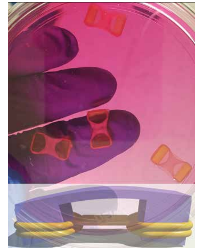
Figure 2: Top view of three thumb-sized biohybrid machines in a culture dish. Modeling and simulations were employed to design and optimize function and performance. These biohybrid machines walk on the dish surface at about one millimeter per second.
