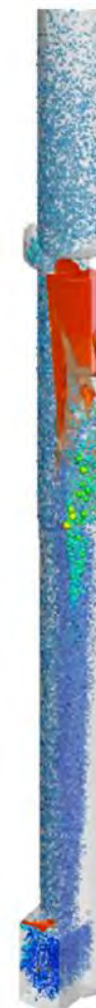
<Predicted argon gas bubbles and gas pocket in a real slide-gate nozzle>
